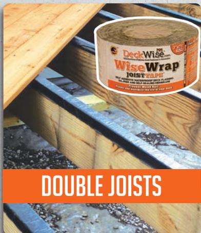
WiseWrap® JoistTape™ is a malleable polyethylene waterproof wood flashing material. It is made of a rubberized asphalt mastic adhesive. Apply to decking joists, around deck support posts and over ledger boards.
